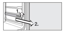
■ To remove a FlexiClip runner so that you can clip it into another shelf runner, for example, lift it at the front and then pull it out along the rail of the oven shelf runner, as illustrated.
